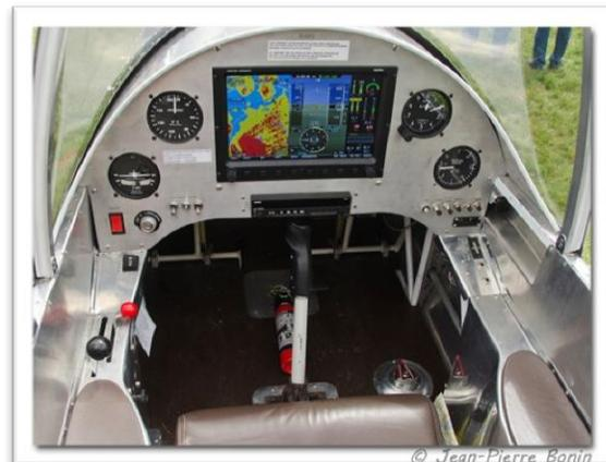
Back in the circuit for some touch and goes. The elevator trim is actuated electrically from a toggle switch on the control stick and the flaps are also electrically controlled. This makes the aircraft very easy to manoeuvre around the circuit. Approach is done at around 65 to 70 mph and landing this aircraft is a real joy. The flight controls are very effective even at very low speed.
